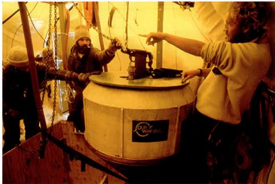
First success: A 1992 US mission used a "gopher" (left) to melt a series of holes to the first P-38. Then the team began a perilous descent.
